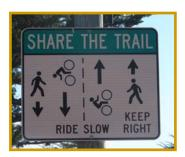
In general, all signs should be located at least three to four (3-4) feet from the edge of the paved surface, have a minimum vertical clearance of eight-and-a-half (8.5) feet when located above the trail surface, and be a minimum of four (4) feet above the trail surface when located on the side of the trail. All signs should be oriented so as not to confuse motorists. The designs (though not the size) of signs and markings should be the same as used for motor vehicles as per the MUTCD.
