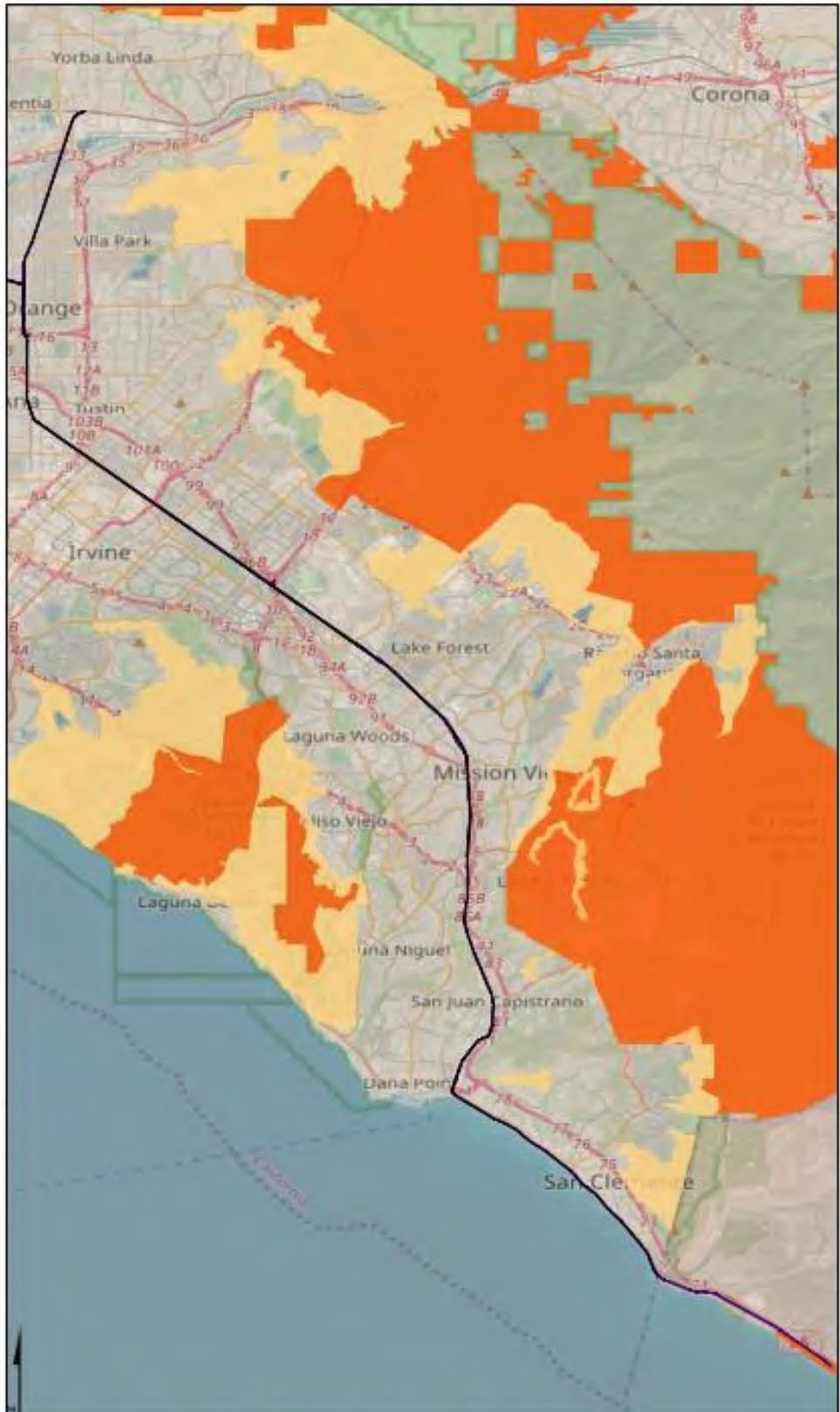
Notes: Asset and centerline data provided by Orange County Transportation Authority. Coastal flooding and cliff retreat data from USGS CoSMoS v3. Inland flooding data from FEMA. Slope failure data from two DEMs: USGS Coastal National Elevation Database and National Elevation Dataset. Heat data from California Heat Assessment Tool. Wildfire data is a summary of three models: MC2-EPA, MC2-University of Idaho, UC Merced.
