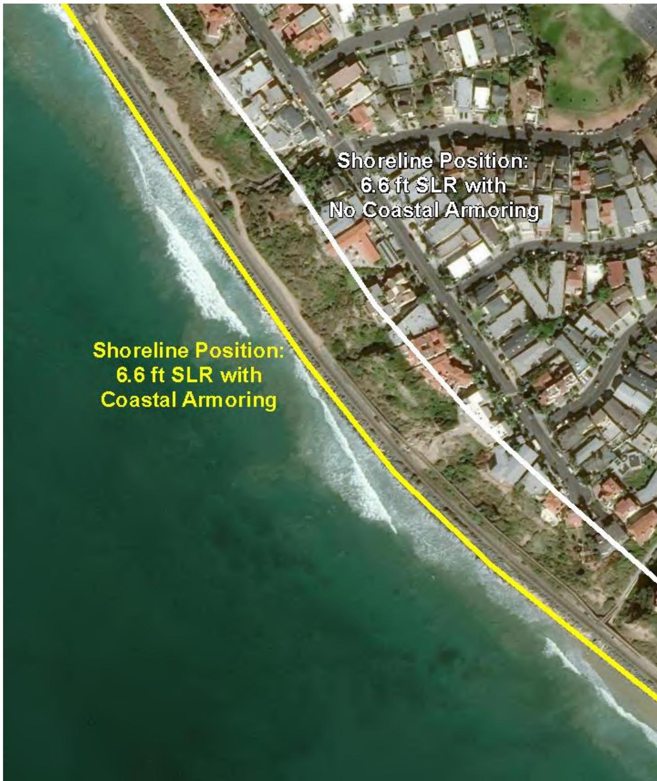
**FIGURE 29 | Shoreline Position with and without Coastal Armoring, 6.6 feet SLR, southern Orange County (USGS CoSMoS)**
