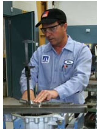
Ray Consiglio checks the internal bearings clearance while performing a transmission rebuild at the Santa Ana Base Maintenance facility.
