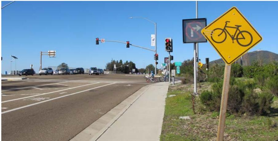
Close up of no-right-turn-on-red signal alerting the driver to wait for a green light.
