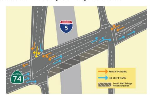
Crews will open the pedestrian walkway on the north half of the Ortega Highway bridge the morning of Sunday, June 2. This walkway was constructed in preparation for the upcoming south half bridge demolition activities. During the south half bridge reconstruction, there will be no pedestrian access on the south side of the bridge. Pedestrians will be directed to utilize the walkway on the north side of the bridge.
