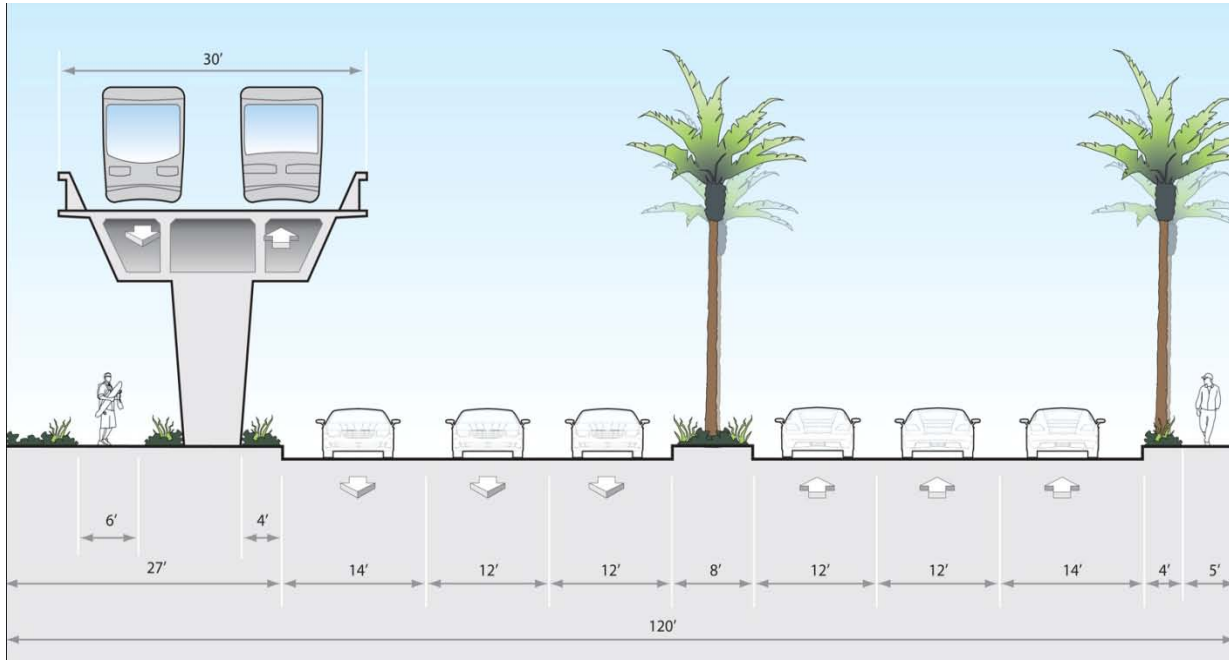
Figure ES.9 – Elevated Fixed-Guideway Alternative: Typical Cross-Sections
