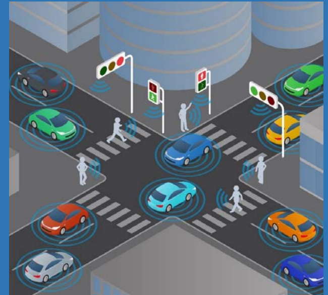
Roadside equipment and standardized in-vehicle devices support V2V and V2I
