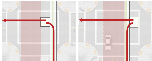
Cycle track turn box protected by physical buffer: Bike lane turn box protected by parking lane:
