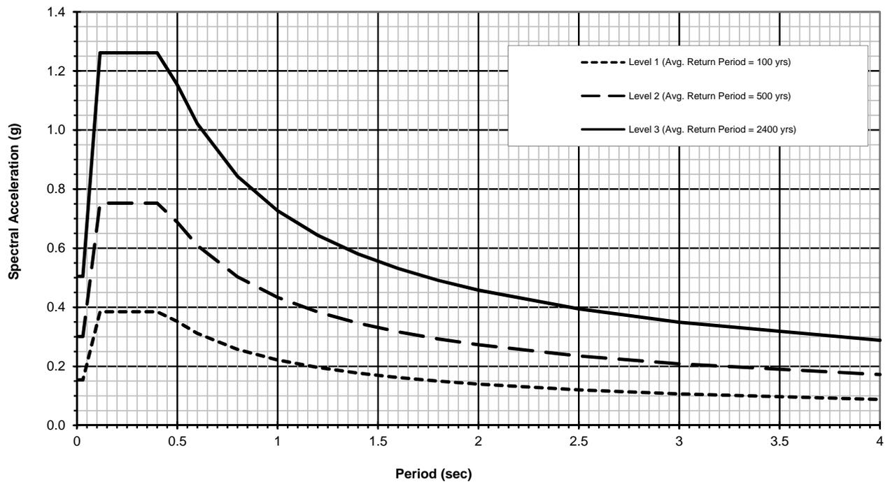
Ref: AREMA (2006) Volume 2 Structures - Seismic Design
