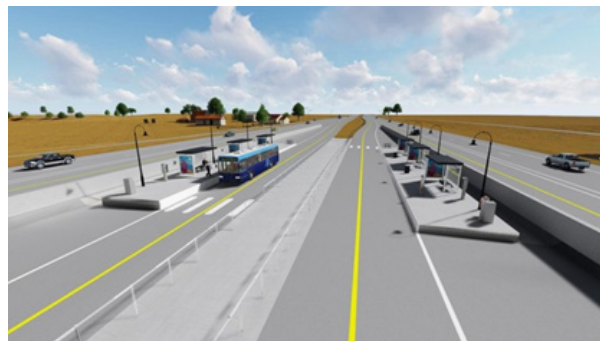
Figure 5: Illustration of the center-load Bustang stop in the middle of I-25, looking north
