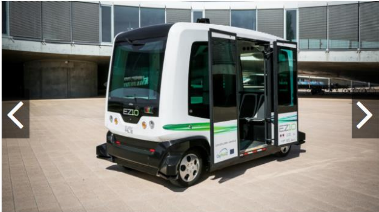
Easymile's EZ10 is a driverless, electric shuttle that can carry up to 12 people.
